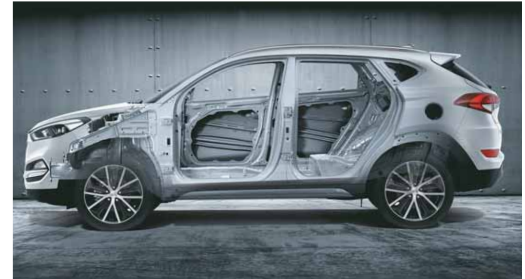
Strong structure with 51% Advanced High Strength Steel
