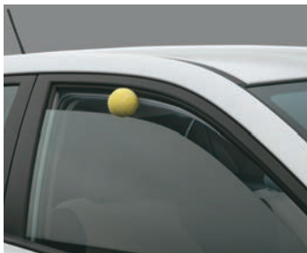
Auto Up/Down Power Window with Pinch Guard
